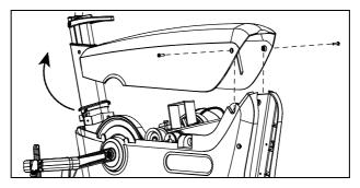
Figure 3: Top cover removal
